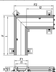
All dimensions in mm and inches. Includes legs, nuts, bolts, and gaskets as shown. If Stainless Steel grade AISI 304 / EN 1.4301 is required specify type no. without suffix S.
