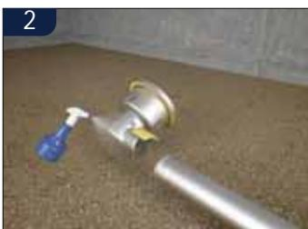
**UK** Wipe the outlet with a cloth and apply lubricant to the outlet for easy assembly.
